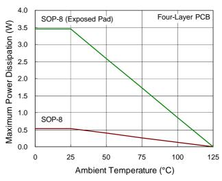
Figure 1. Derating Curve of Maximum Power Dissipation
