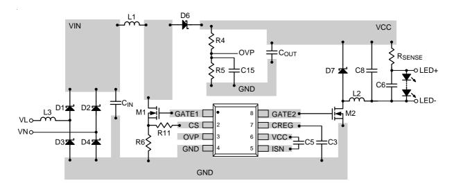
Figure 2. PCB Layout Guide for SOP-8 Package
