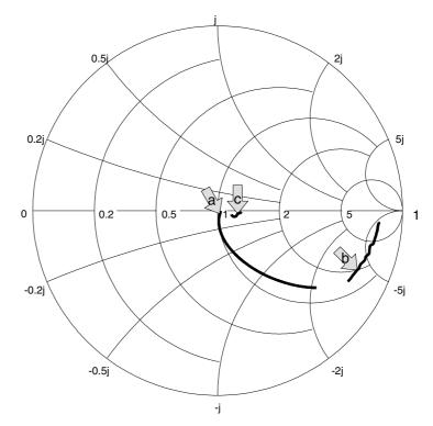
a: LO input, LO frequency from 100 MHz to 1100 MHz, marker: 950 MHz b: RF input, RF frequency from 100 MHz to 1100 MHz, marker: 950 MHz c: I/Q Outputs, Baseband Frequency from 5 MHz to 55 MHz, marker: 25 MHz
