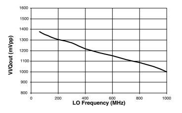
Figure 6-8. Typical Suitable LO Power Range versus Frequency
