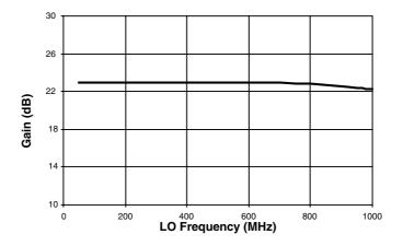
**Figure 6-7.** Typical Output Signal versus LO Frequency for  $P_{RF} = -15$  dBm and PLO = -15 dBm
