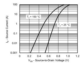
Source-Drain Diode Forward Voltage
