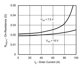
On-Resistance vs. Drain Current
