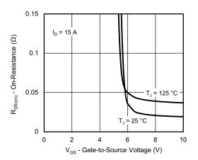
On-Resistance vs. Gate-to-Source Voltage
