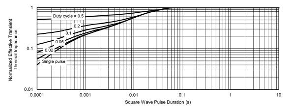
Normalized Thermal Transient Impedance, Junction-to-Case
