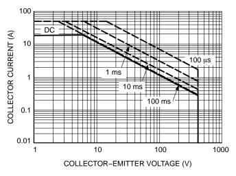
Figure 13. Single Pulse Safe Operating Area (Mounted on an Infinite Heatsink at  $T_A = 25$ °C)
