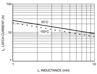
Figure 10. Minimum Open Secondary Latch Current vs. Inductance
