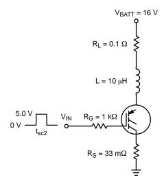
Figure 18. Circuit Configuration for Short Circuit Test #2
