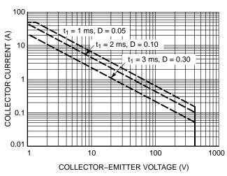
Figure 16. Pulse Train Safe Operating Area (Mounted on an Infinite Heatsink at  $T_C = 125^{\circ}C$ )
