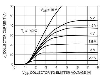
Figure 2. Output Characteristics
