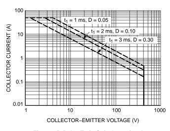
Figure 15. Pulse Train Safe Operating Area (Mounted on an Infinite Heatsink at  $T_C = 25^{\circ}C$ )
