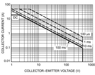
Figure 14. Single Pulse Safe Operating Area (Mounted on an Infinite Heatsink at  $T_A = 125$ °C)
