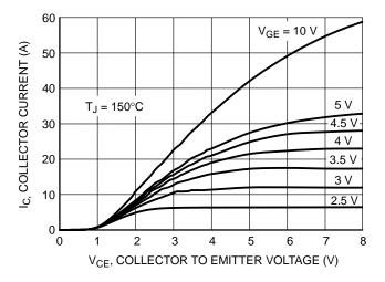
Figure 3. Output Characteristics
