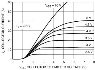
Figure 1. Output Characteristics
