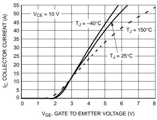
**Figure 4. Transfer Characteristics**
