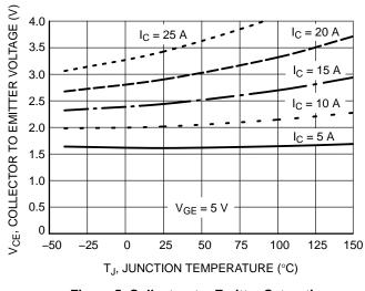
Figure 5. Collector-to-Emitter Saturation Voltage vs. Junction Temperature
