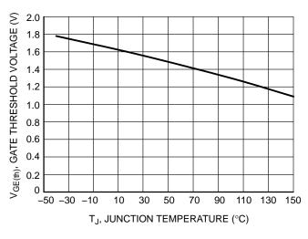
Figure 9. Gate Threshold Voltage vs. Junction Temperature
