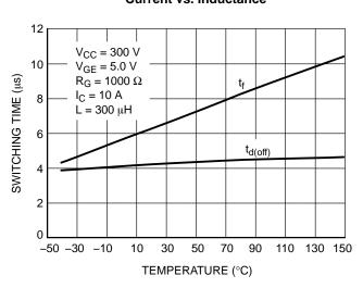
Figure 12. Inductive Switching Fall Time vs.
