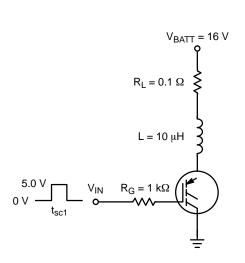
Figure 17. Circuit Configuration for Short Circuit Test #1
